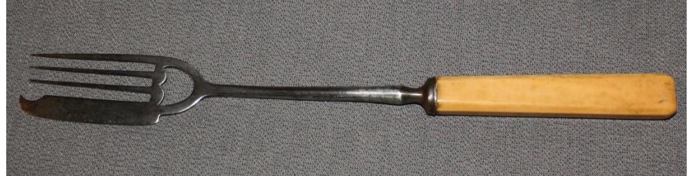
Attachable eating utensils for arm prosthetics
